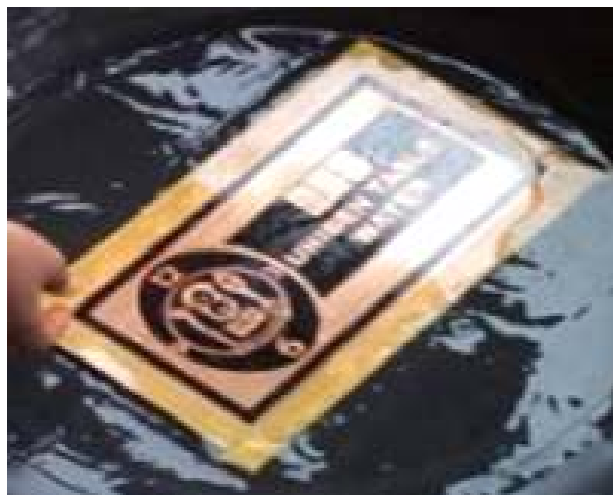
Plate 8 inserting the copper plate with design in the prepared solution for etching process to commence Photo: Samson Ukweku, 2020
