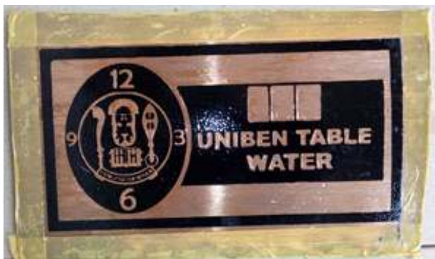
Plate 6: Transferred design on a copper plate through screen printing method. Photo: Samson Ukweku, 2020
